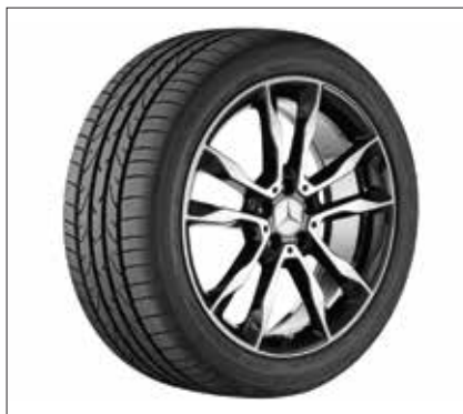
5-twin-spoke wheel | Black, high-sheen Wheel 8 J x 19 ET 43.5 | Tyre 235/45/R19
